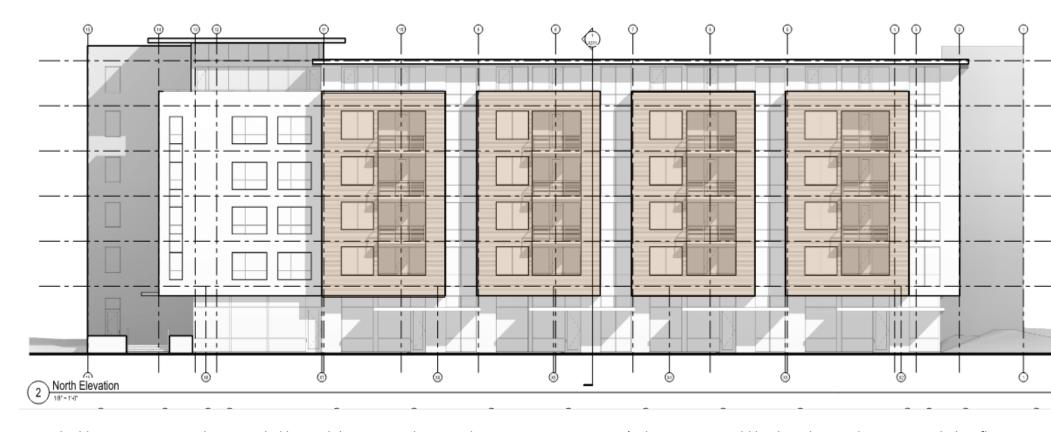
A past build in our juristiction that extended beyond the property line into the ROW IBC 3202.3 over 8'. The concern would be the substantial structure including floor area, respectively.
