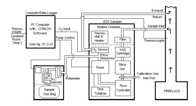
Figure 31-2-1. Schematic of ESS/Data Logger system.
