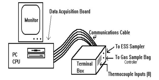
Figure 31-2-2. ESS data logger system.
